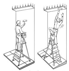
Always remain centered on the equipment. Stretching or reaching can cause you to lose balance and fall.
